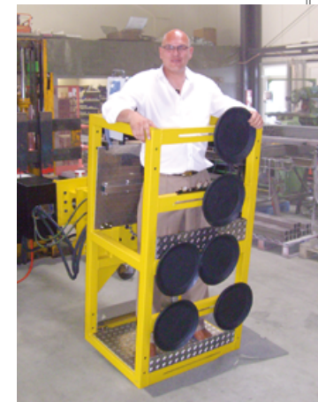
Workman's basket with suction system
