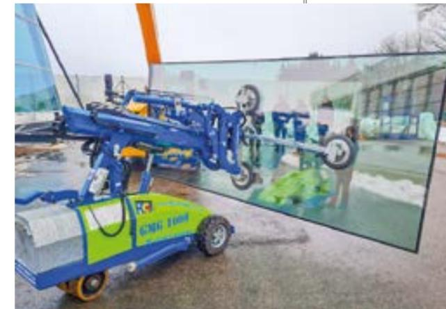
The GMG 1000 glass assembly device was used to transport the 800-kilo glass pieces. This equipment allows panes weighing up to 1000 kilos to be safely transported indoors and outdoors by just one installation engineer, even in confined spaces or through narrow passageways.
